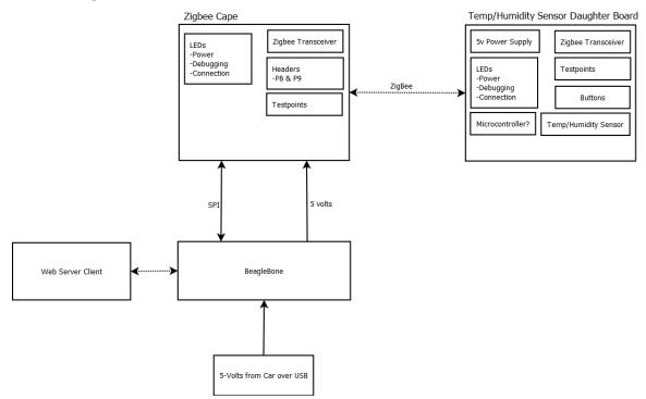
This schematic shows how our cape connects to the beaglebone, and how wireless communication is handled.
